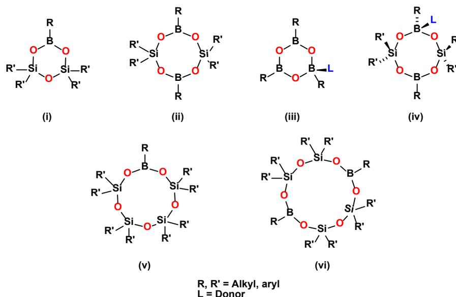
**Figure 1.** Structures of (i) 6-membered cyclo-boradisiloxane; (ii) 8-membered cyclo-diboradisiloxane; (iii) 1:1 adduct of a boroxine; (iv) 1:1 adduct of a cyclo-diboradisiloxane; (v) 10-membered cyclo-diboratetrasiloxane; (vi) 12-membered cyclo-diborahexasiloxane.
