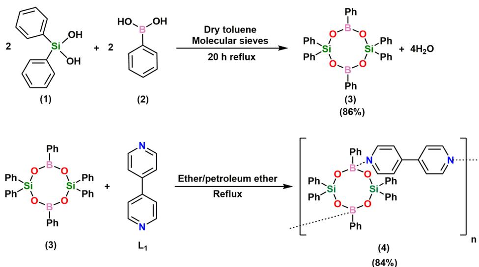
**Scheme 1.** Preparation of (Ph<sub>6</sub>B<sub>2</sub>Si<sub>2</sub>O<sub>4</sub>) (3) and [Ph<sub>6</sub>B<sub>2</sub>Si<sub>2</sub>O<sub>4</sub>]-L<sub>1</sub> (4) adduct.
